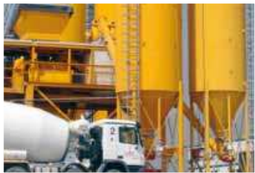
Ready-mix concrete production
